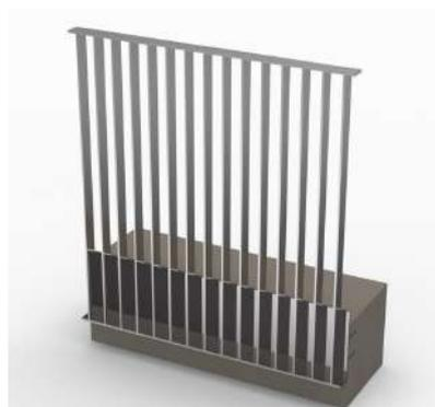
All 50x8mm flat bar with a continuous side mounting plate (300x10mm)
