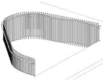
Meridan is a mixed hardwood balustrade on a steel edge plate.
